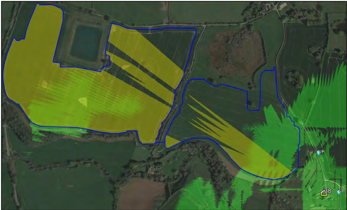
Figure 27 Visible terrain (green areas) for an observer at 2m above ground level at dwelling 38
