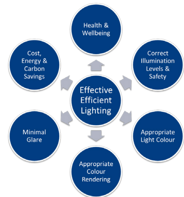
Figure 26: Effective and efficient lighting design needs to take into account a wide range of factors
