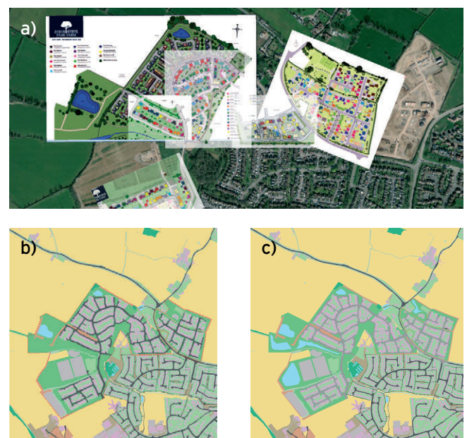
Figure 5: (a) Map of an example housing development overlaid onto an aerial photograph. (b) Our digital approximation of the proposed housing development. (c) A scenario where we have introduced ponds (shaded in blue) in public greenspaces > 300 m 2 .
