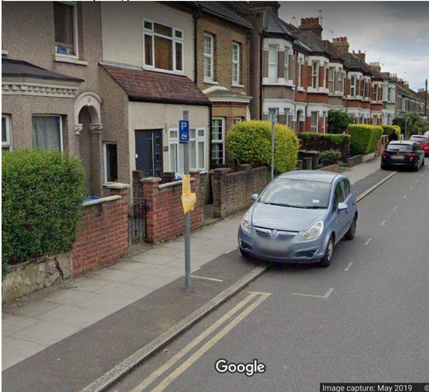
Figure 1. A residential London street with an exemption from the London-wide pavement parking prohibition. Upright traffic signs show the start and end of permitted pavement parking, and white bay markings show how much of the pavement drivers may occupy.
