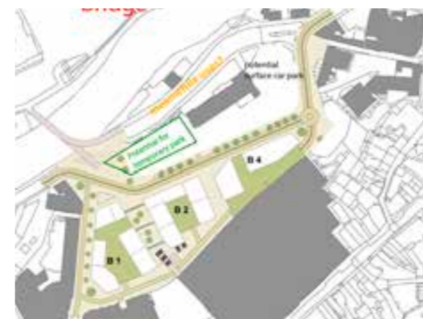
phase 3 redirection of traffic onto New Smithfield Road enables construction of Smithfield Gardens and remaining blocks.
