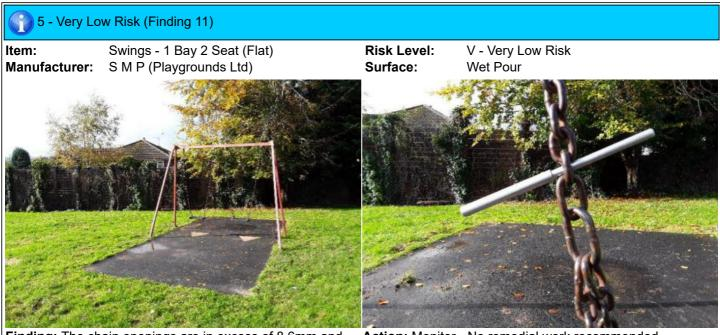
**Finding:** The chain openings are in excess of 8.6mm and do not meet the recommendations of BS EN 1176 Part 1
