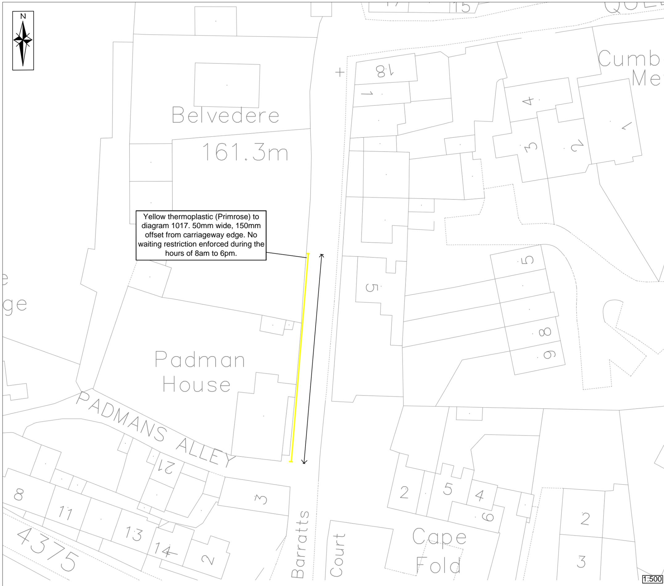
Yellow thermoplastic (Primrose) to diagram 1017. 50mm wide, 150mm offset from carriageway edge. No waiting restriction enforced during the hours of 8am to 6pm.
